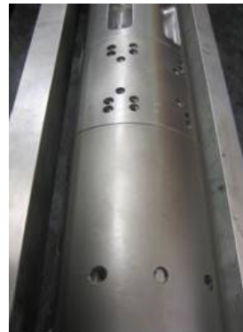
Figure 17: Wet Connector Mated on test Rig
