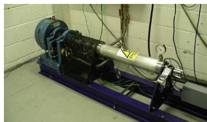
Figure 11a – the 1 st generation motor test bed (limited to 60°C water temperature)
