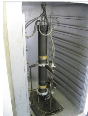
Figure 14: Wet Connector Testing lab (Oven closed, control valve manifold visible on outside)
