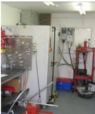
Figure 13: Wet Connector in pressure Test Vessel in Oven
