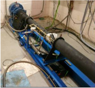
Figure 11b – the 2nd generation motor test bed (180C testing temperature)
