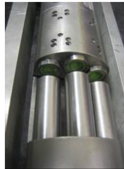
Figure 16: Wet Connector De-Mated on Test Rig
